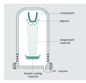
surfaces because of an electrical potential difference. A common term for the trajectory for this type of deposition is "line of sight" and so the process is most useful for simple geometries.
