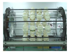
a few small parts are in the chamber at a time. This permits a vacuum to be drawn much more quickly, and the metallization of small parts using such a system can be in-line, synchronous with other operations such as molding, or coating.
